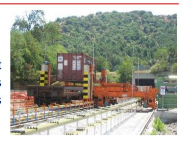
A key feature of the Metrocargo® system is its adaptability to any kind of train and container type WITH NO NEED OF SPECIAL MODIFICATIONS TO THE WAGONS NOR THE CONTAINERS. Optical recognition technology allows the system to "read" a train composition as it enters the station and even the identifiers of each single container (no need of special RFID or barcoding).
