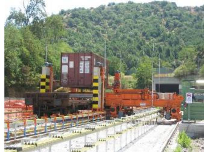
A key feature of the Metrocargo® system is its adaptability to any kind of train and container type WITH NO NEED OF MODIFICATIONS TO THE WAGONS NOR THE CONTAINERS. Optical recognition technology allows the system to “read” a train composition as it enters the station and even the identifiers of each single container (no need of special RFID or barcoding).
