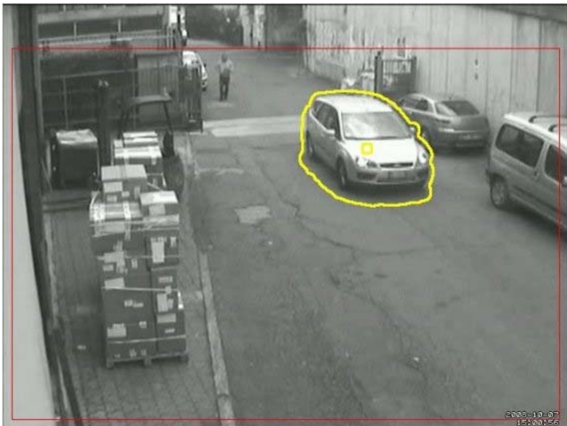
Figure 6 – A car is approaching correctly classified as a rigid object
