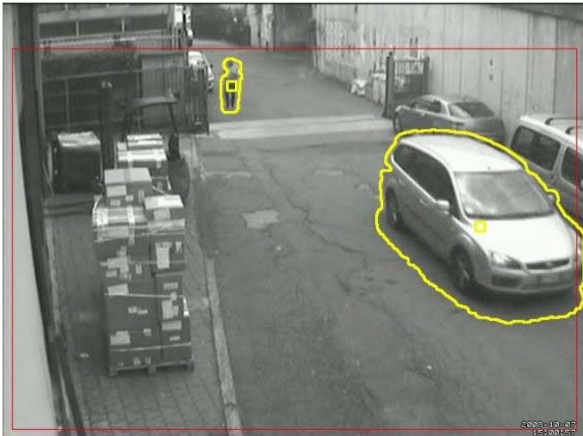
Figure 7 – A person walks frontally towards the camera and for a while it is recognised as a rigid object
