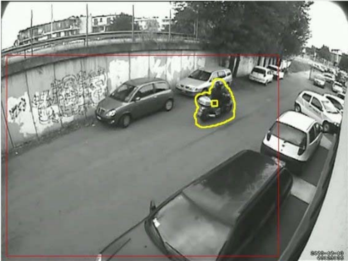
Figure 5 – A motorbike passes ride by a person: the object is rigid and the algorithm correctly classified it
