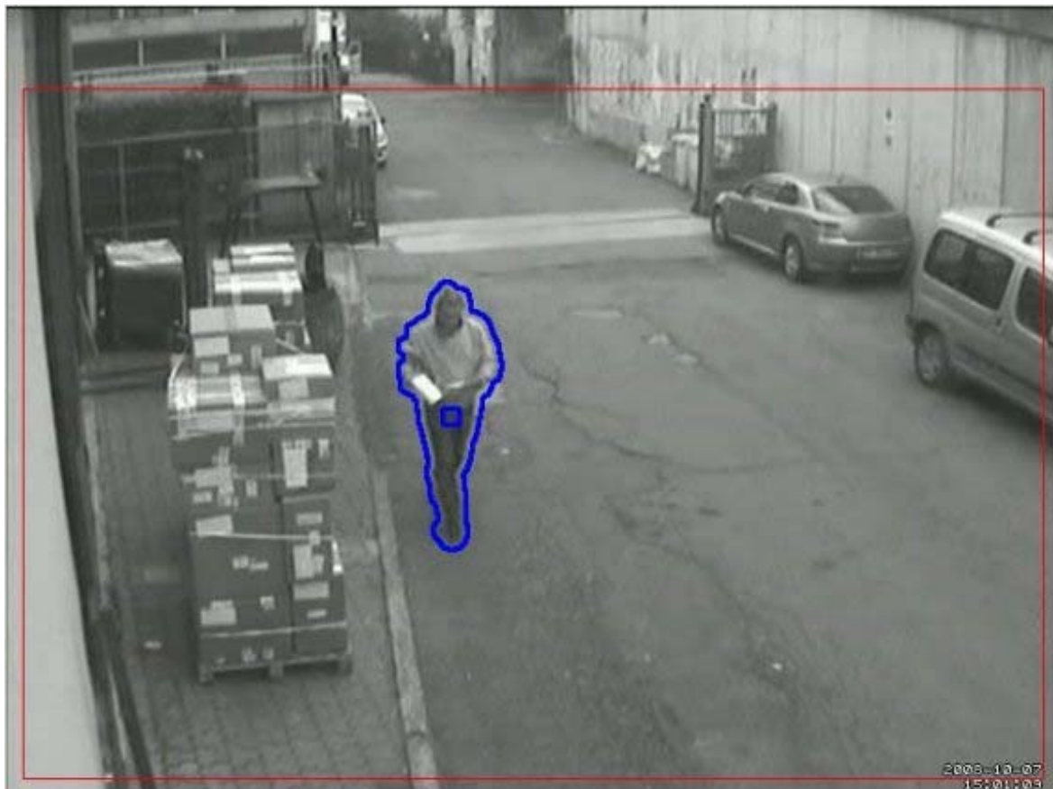
Figure 8 – The person gets near to the camera and the algorithm correctly classifies it as a non-rigid object
